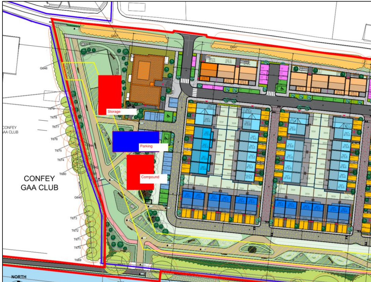
Figure 3: Construction Site Compound
