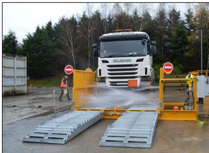
Figure 7: Example Wheel Wash System
